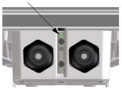
Note The LED is only in use until installation is completed, and is **automatically disabled** 10 minutes after the connection is established. After this, the LED is only active during reboot of the EXPLORER 540 or if you restart the installation process.
