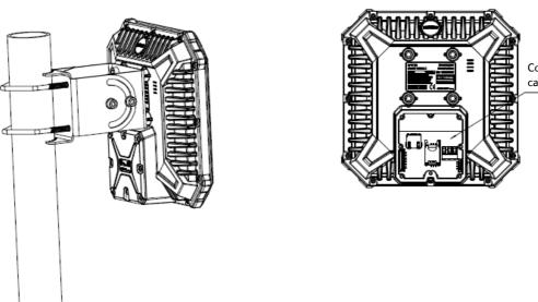
Compartment for SIM card and connections
