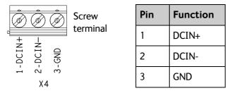
To unscrew and fasten the screws in X4 use a screwdriver (max. 3.5 mm wide). If the DC cable is shielded, connect the shield to pin 3, GND. Otherwise leave GND unconnected.
