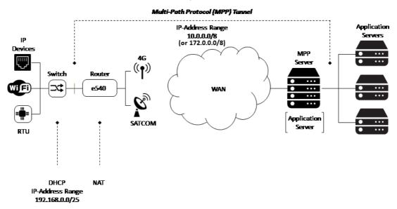
To set up PRISM you must install the PRISM server software from Cobham SATCOM, configure the PRISM server and set up your EXPLORER 540 to communicate with this server.
