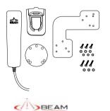
Mount the handset cup to the mounting plate, it can be installed to the left or right side of the dock by simply rotating the bracket.
