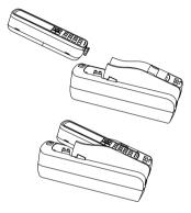
To remove the handset from the cradle, press the EJECT button at the top of the docking station. The dock will swing out and the handset can be removed.
