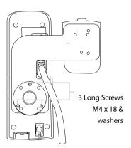
Plug the Privacy Handset RJ9 connector into the bottom of the docking unit, as per image below. Privacy Handset mode is enabled when the handset is removed from the cup. Please ensure to re-dock the Privacy Handset when not in use.
